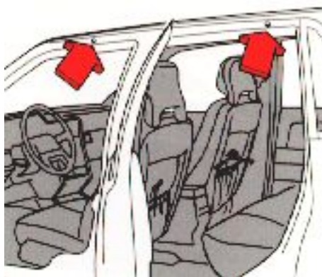
Holes for roof rack
