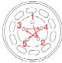
Correct tightening order for wheel bolts
