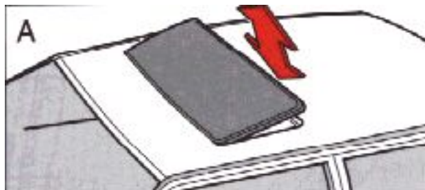
A- Ventilation position
